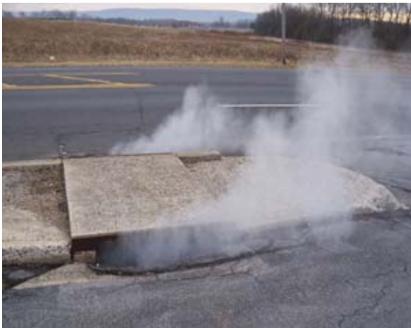
Smoke exiting storm drain
